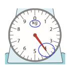
The needle is pointing towards 4 on the scale. We can see that we are measuring mass using kilograms (this is underneath the 0). The watermelon weighs 4kg. We say this as four kilograms.
